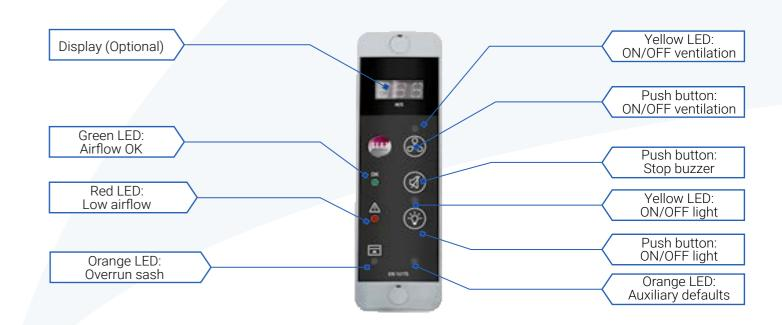
The TYPE C remote HMI controller is a safety device for controlling the ventilation of a fume hood using a PID controller. It adjusts the ventilation to maintain the set speed regardless of the height of the glass. Visual and audible alarms alert the user if a malfunction occurs.
