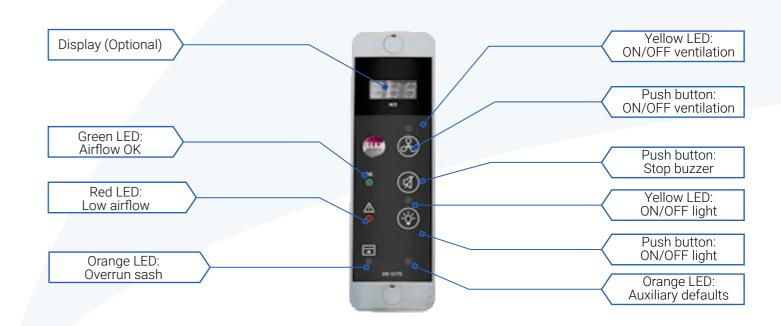
The TYPE C 2-speed remote HMI controller is a safety device that regulates the airflow according to a low and high speed depending on the sash position. The controller engages the second speed by means of a switch placed on the sash path. It informs the user with visual and audible alarms if a malfunction occurs. The remote HMI enables adjustments on site and controls the fume hood ventilation.
