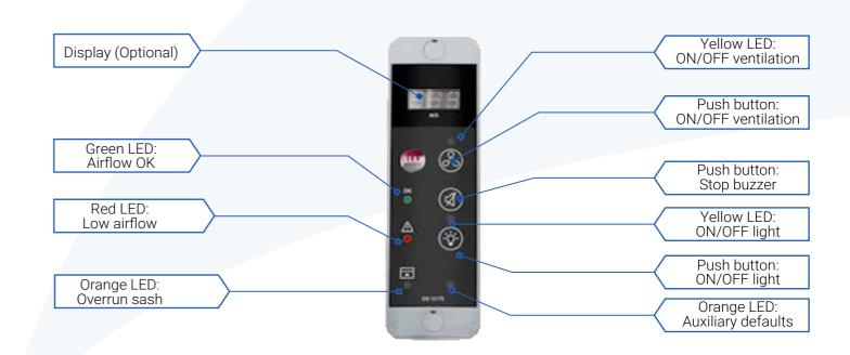
The type A remote HMI controller is a safety device which monitors the fan connected to a lab fume hood. A speed sensor measures the face velocity and built in visual and audio alarms alert the user in the event of any malfunctions. On-site adjustments are possible.
