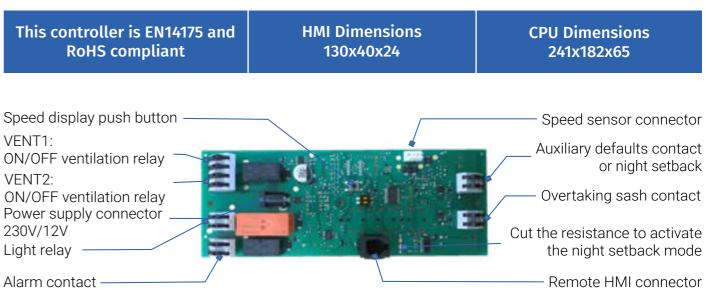
VENT1: ON/OFF ventilation relay VENT2: ON/OFF ventilation relay Power supply connector 230V/12V Light relay
