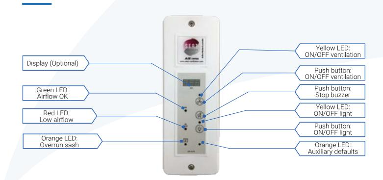
The TYPE A controller is a security device which monitors the fan from a lab fume hood. A speed sensor measures the face velocity. It informs the user with visual and audible alarms if a malfunction occurs. On-site adjustments are possible.
