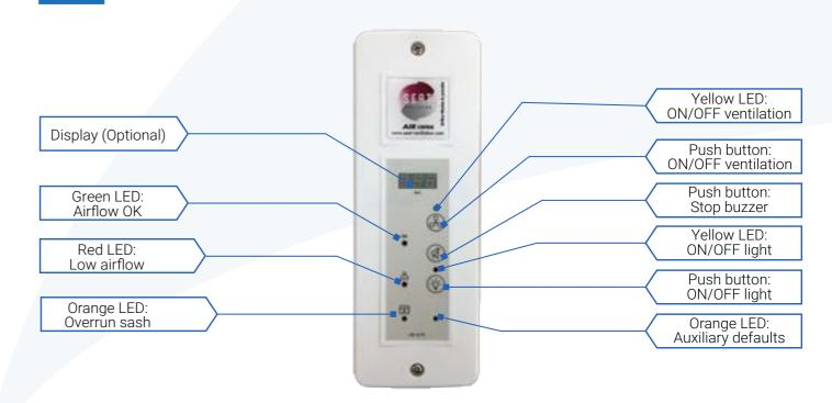
The TYPE C controller is a safety device for controlling the ventilation of a fume hood using a PID controller. It adjusts the ventilation to maintain the set speed regardless of the height of the glass. It informs the user with visual and audible alarms if a malfunction occurs. The remote HMI enables adjustments on site and controls the fume hood ventilation.
