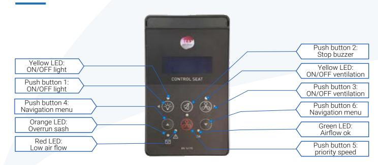
The CONTROL SEAT is a safety device for controlling the ventilation of a fume hood. It adjusts the ventilation to maintain the set speed regardless of the sash height. It informs the user with visual and audible alarms if a malfunction occurs. The remote HMI enables adjustments on site and controls the fume hood ventilation. It has many operating modes and can be combined with a linear position sensor.
