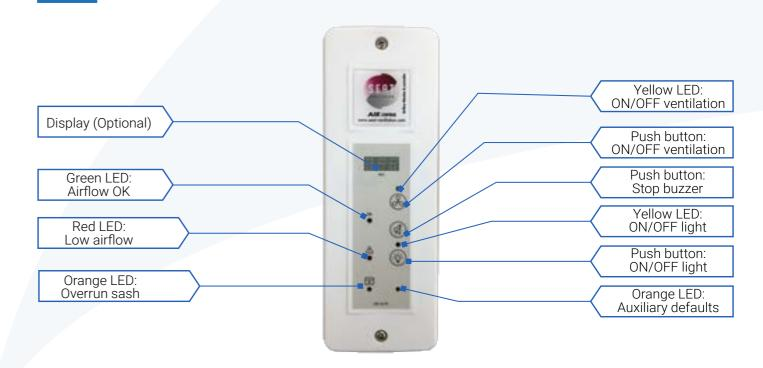
The TYPE C 2-speed controller is a safety device that regulates the airflow according to a low and high speed depending on the sash position. The controller engages the second speed by means of a switch placed on the sash path. It informs the user with visual and audible alarms if a malfunction occurs. The remote HMI enables adjustments on site and controls the fume hood ventilation.
